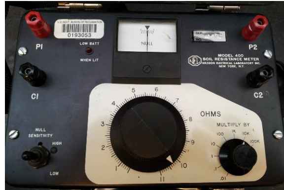
Figure 58. Meter for determining resistivity of soil around anodes.
