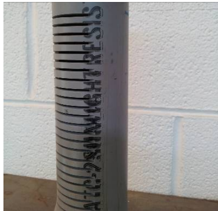
Figure 14. Conduit for mounting submerged anodes such as rod and wire anodes. Note the slots are only over 180 degrees of the circumference on one side of the pipe.
