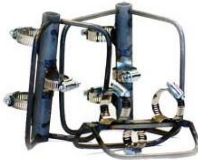
Figure 23. Example of device for centering anodes in deep well anode beds. Vent pipe can also be attached to the centralizer for easier installation. (Courtesy of Brance-Krachy Co., Inc.)
