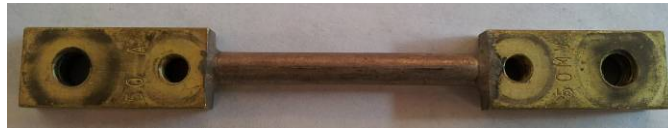
Figure 5. Rectifier shunt for determining current output. Shunt has a rating of 50 amperes/50 millivolts.
